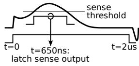
comparator will fire. We OR the two to detect pulses of either polarity. The threshold of 20 mV was chosen by experiment.
