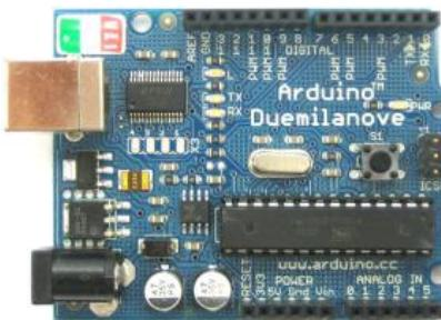
**The Arduino is a popular, easy-to-use, open design microprocessor board with IO capabilities.**
