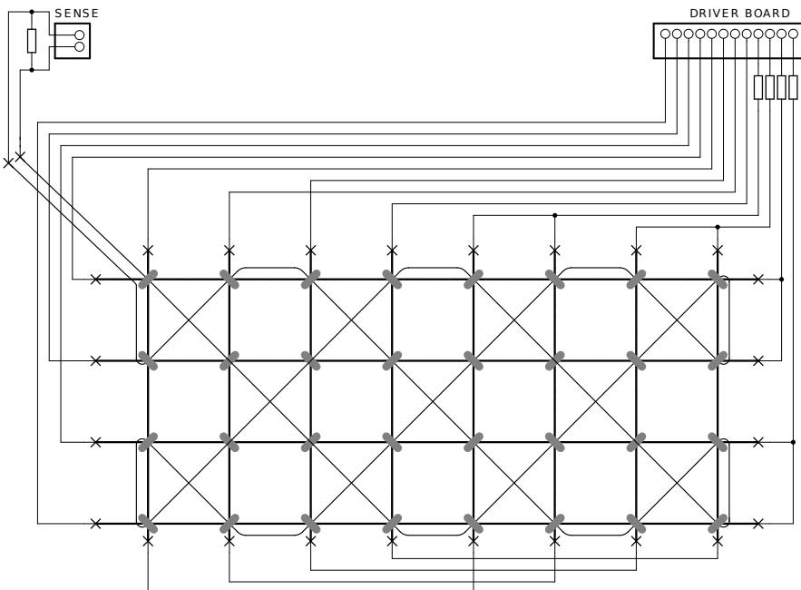
The terminating resistor across the sense loop provides a path for the current caused by the induced voltage round the loop.
