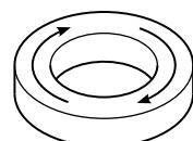
A strong field in the same direction as the core's existing magnetisation has no lasting effect — the core is *saturated* and can be magnetised no further in that direction.
