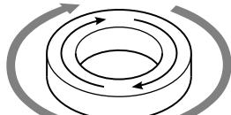
*When this external field is removed, the magnetism in the core reduces slightly in strength, but remains clockwise:*
